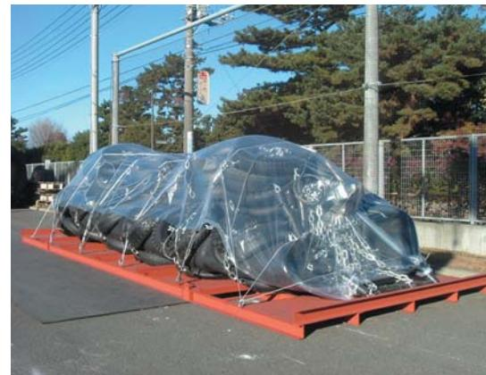
Fig.3-15 Vacuumed and Folded Down Condition for  $\phi 4500 \times 9000L$ -P80
