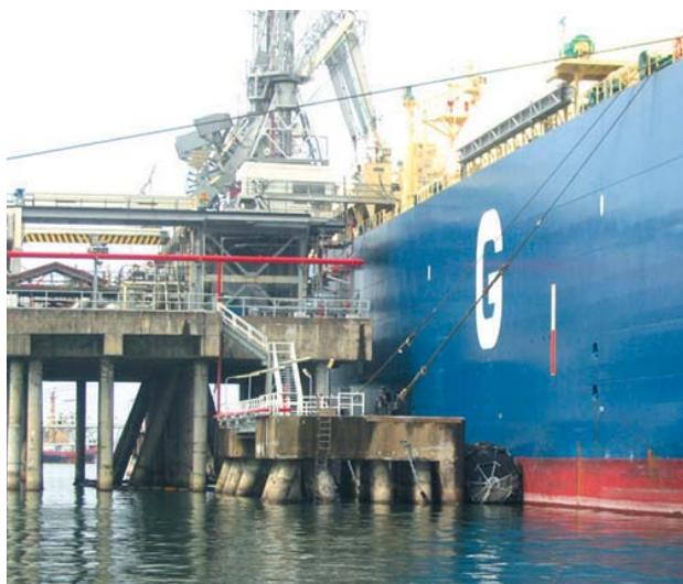
Fig.3-7 Yokohama Pneumatic Fender φ3300×6500L
