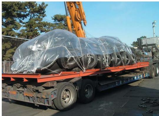
Fig.11-1  $\phi 4500 \times 9000\text{L-P}80$  Transportation on Steel Pallet
