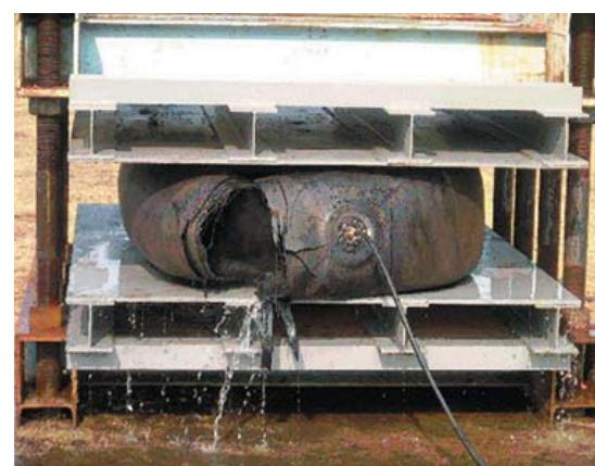
Fig.3.3 Burst Test at 60% Deflection
