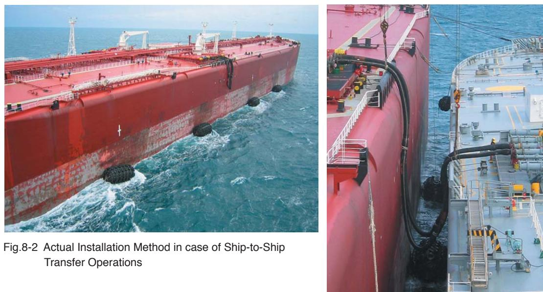
Fig.8-2 Actual Installation Method in case of Ship-to-Ship Transfer Operations
