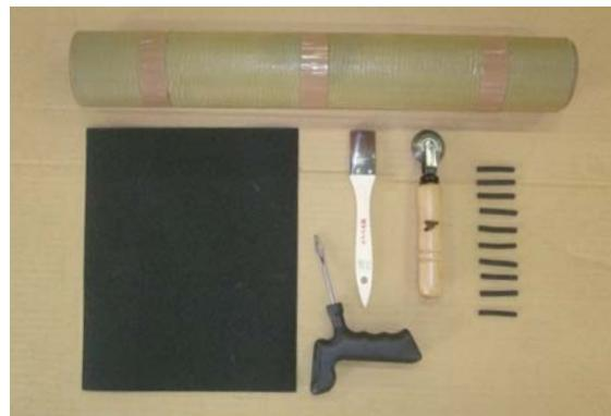
Repair Tool Kit for Small and Medium size Fenders
